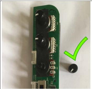
Re-install your new PT01 Scratch Control Assembly Board.
