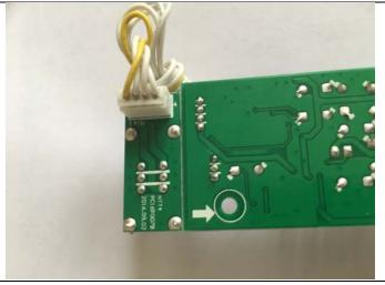
Turn the board over, un-wind the white 'ribbon' cable and snap off the surplus switchboard, which can be disposed of. Take off all three of the rotary knobs from your damaged/faulty board and place on the new PT01 Scratch Control Assembly Board.
