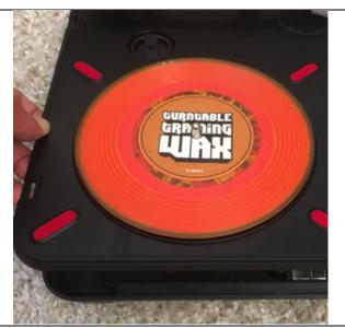
4 Use a small flathead screwdriver to help lift the felt from the side directly opposite from the cartridge and needle.
