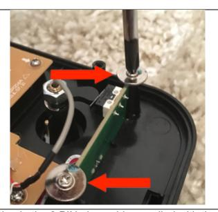
Plug in the 2 PIN plug cable supplied with the new Latching Relay into the relays plug. Using the newly prepared TE5 power connection from Step 8, connect the red cable into the Latching Relays 'NO' terminal and the white cable into the Latching Relays 'COM' terminal. Slide the Latching Relay into the same post slot assigned for the old Tone Arm Relay. Secure lighly with the washer screws to hold in place.
