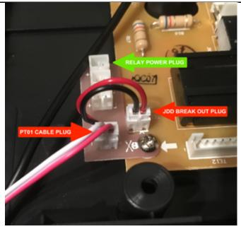
Now tidy up the cabling with either tape or hot clue, put it back together by repeating Step 1 in reverse. If the start stop fails to work, **ensure all cable connections are making contact.**
