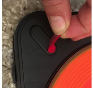
Once the priming hole is large enough for the step drill bit, start drilling slowly, with slight pressure through the table top. The required 30mm hole need will take you to the very last
