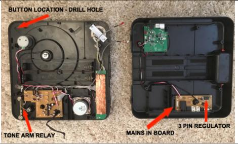
Remove the top cover and place the turntable upside on top, in order to have a catchment area for plastic drilling debris. Ensure it is loose so when drilling, you are able to lift up the table top and to stop the drill bit continuing through the top cover.
