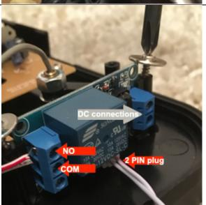
10 Connect the Latching Relays 2 PIN plug cable open ends to the 'terminal connection block' from the white taped cable extension. It is good practice to connect the 'red to red' and the 'white to white'. The button is now connected to the Latching Relay.
