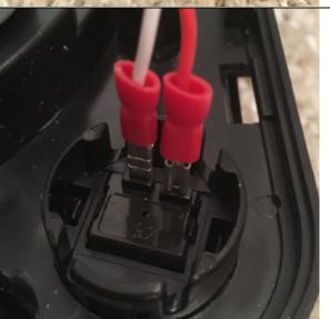
Unscrew the washer connectors from the Tone Arm Relay and lift out the relay from the posts. Cut the power TE5 connection from the relay, right up to the plug. Then, prepare the cable ends with a cable stripper, cable snips or a knife. You only need 0.5cm of bare copper wire showing. Once prepared, twist the wire ends – ready to connect.
