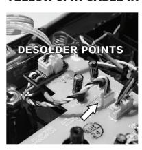
22. ATTACH TONE ARM WIRES IN WITH SMALL FLAT SCREW DRIVER.
